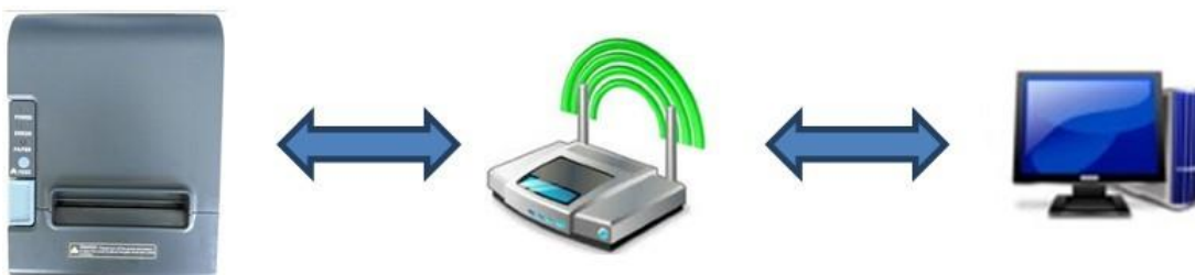
Exemplo 2: IP TP-650 192.168.0.180...IP Roteador 192.168.0.1.....IP Computador 192.168.0.150
